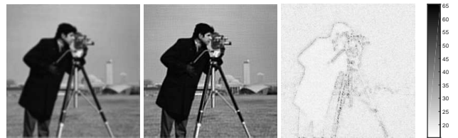
Fig. 6. Image deblurring with wavelets. Noisy and blurred observation (left), MMSE estimate \mathbf{W}\hat{\mathbf{x}} (middle, SNR = 21.52 dB) and 90% credibility intervals computed with SGS (right).
